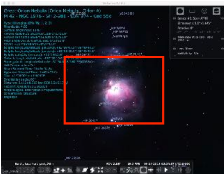
Orion Nebula (M42) with C90 1250 mm Telescope, Full Frame Camera, FOV 2.88 degrees
